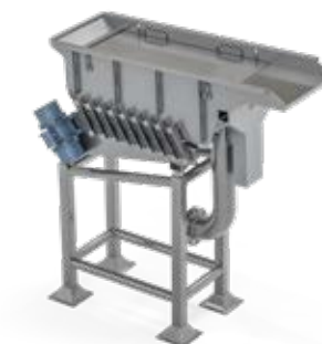
SLICE PREPARATION The slice is gently washed in mechanical vibrating system.
