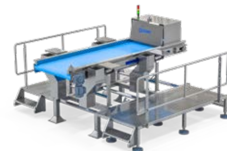
INSPECTION STATION Conveyor (manual inspection)
