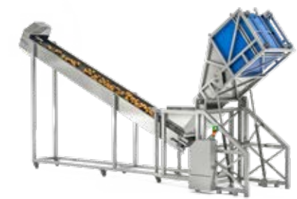
POTATO RECEIPT AND FEEDER Raw potato receipt by hydraulic lifting system.
